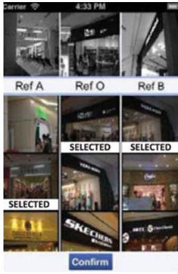
Fig. 17. The UI presented to the user for correction of image matching results. The top row are the three test images taken by the user, below each are the top 3 matched reference objects. The user can denote the correct match by tapping the thumbnail images.
