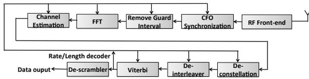
Figure 1: Illustration of the 802.11a/g PHY receiver
