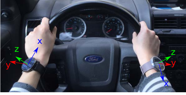
Figure 2: The 3-axis coordinate system for the accelerometers and gyroscopes on the smartwatches. The most important fact is, the X-axis is always parallel to the arm, and its direction for the left and right arm is opposite to each other.
