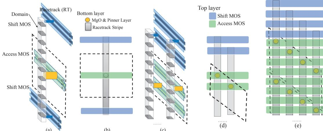
Fig. 3. The layouts of macro unit (MU). (a) Side view of one cell MU layout. (b) Top view of one cell MU layout. (c) Side view of MU layout for overlapped cells. (d) Top view of MU layout for overlapped cells. (e) Top view MU layout of four overlapped cells.
