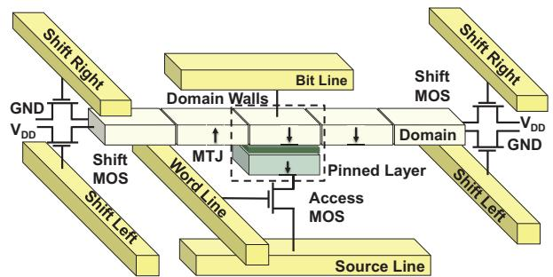
Fig. 1. An illustration of racetrack (RT) structure.
