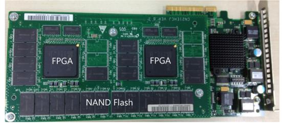
Fig. 5. Prototype of Active SSD.
