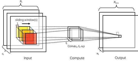
Figure 5. Convolution layer architecture.  $f_i \times f_i$  windows are sliding across the input feature maps.
