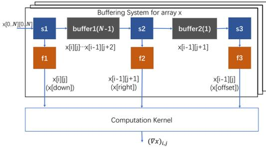
Figure 4. Micro-architecture for TV calculation. Grey, blue, and orange boxes denote buffers, data path splitters and filters, respectively.
