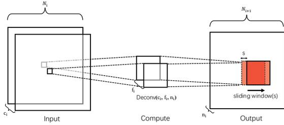
Figure 6. Deconvolution layer architecture.  $f_i \times f_i$  windows are sliding across the output feature maps.
