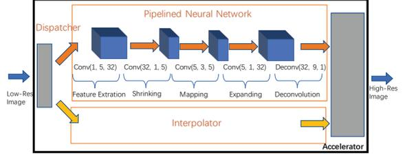
Figure 2. An overview of the proposed system. Grey boxes indicate the input and output frame buffers. The dispatcher is integrated into the input buffer.
