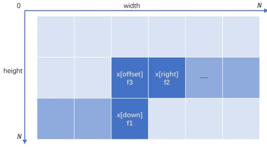
Figure 3. Stencil access pattern of TV computation. Gradients at *offset* rely on the dark blue pixels.
